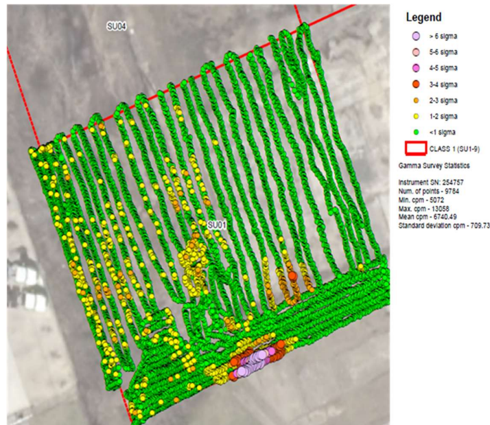
Figure 1. Track of survey unit scans. Count rates as related to the mean are listed in the Legend.
